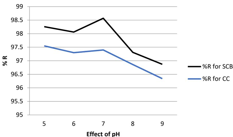
**Fig. 4: Effect of pH on MB adsorption with SCB and CC**
