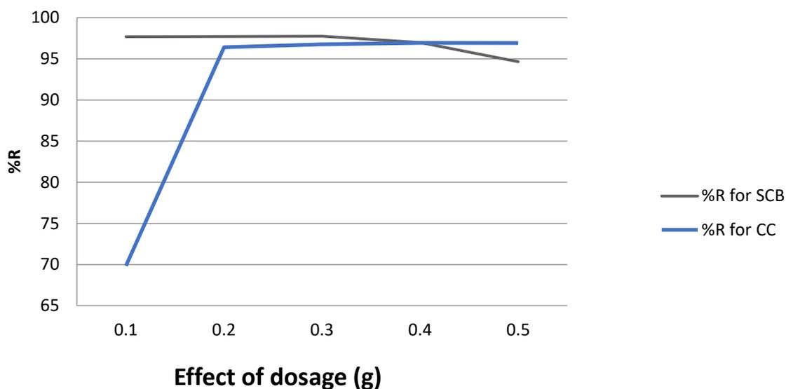
**Fig. 1: Effect of SCB and CC dose on MB adsorption**
