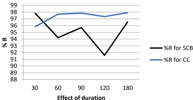
**Fig. 2: Effect of duration on MB adsorption with SCB and CC**
